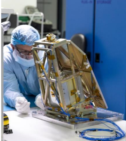
MSolo mounted on its vibration test fixture during verification and validation testing at KSC
